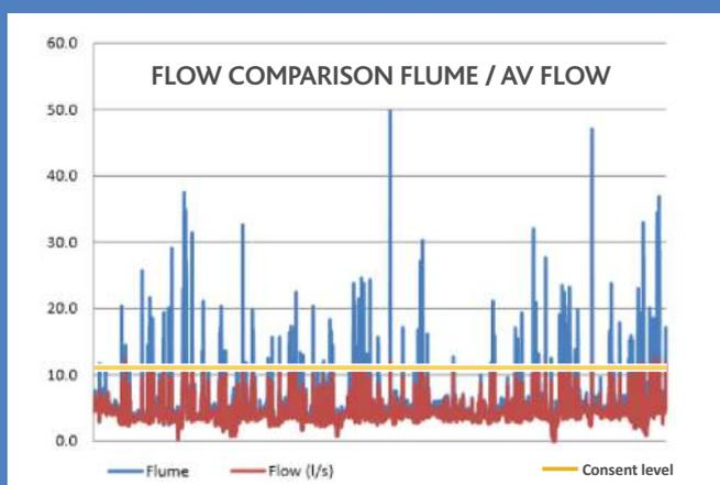
The graph shows a vast, consistent breach of consent when using data from the primary flow measurement, which is not the case when using data from the **MSFM**.
